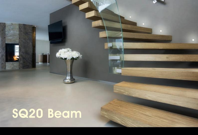
In contrast to the glare-free SQ20 Mosaic, the SQ20 Beam has a clear surface with light guide fins and is therefore significantly brighter. It is used wherever a higher luminous efficacy is expressly desired, for example as lateral staircase lighting.
